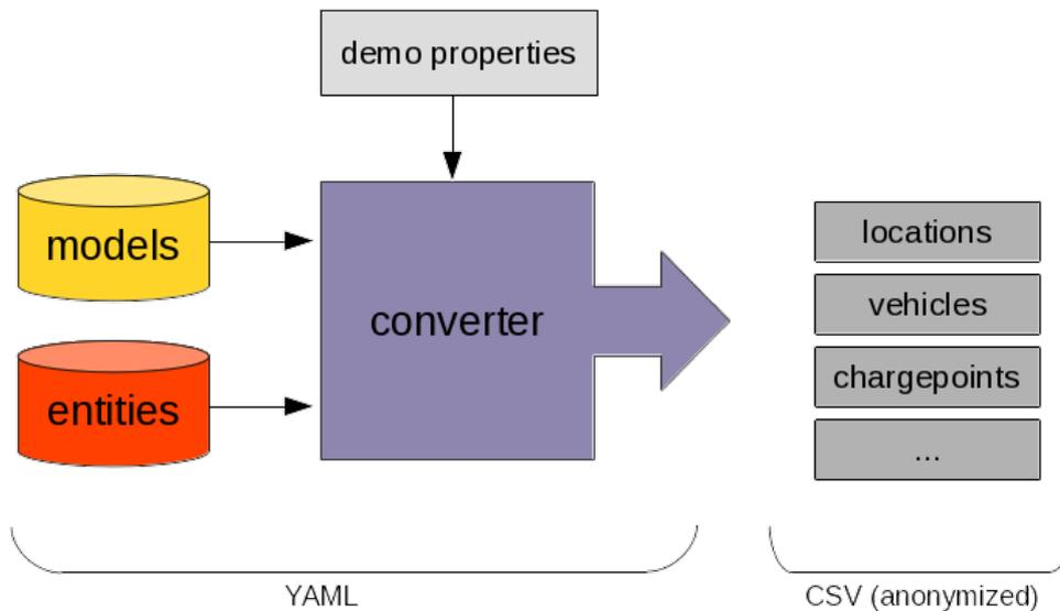
**Figure 2 - Converter Software workflow merging multiple device and model files**
