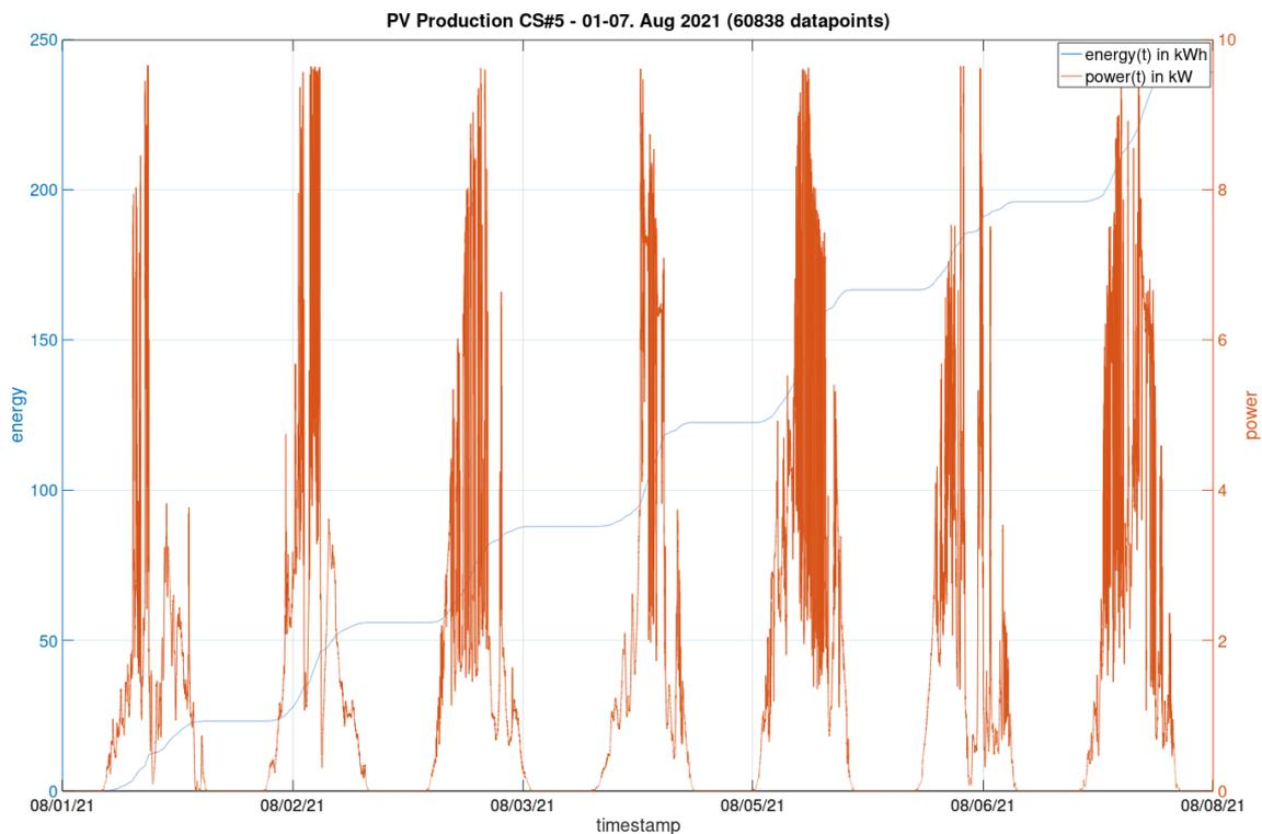
**Figure 13 – PV energy production chart from CS#5 (7 days)**
