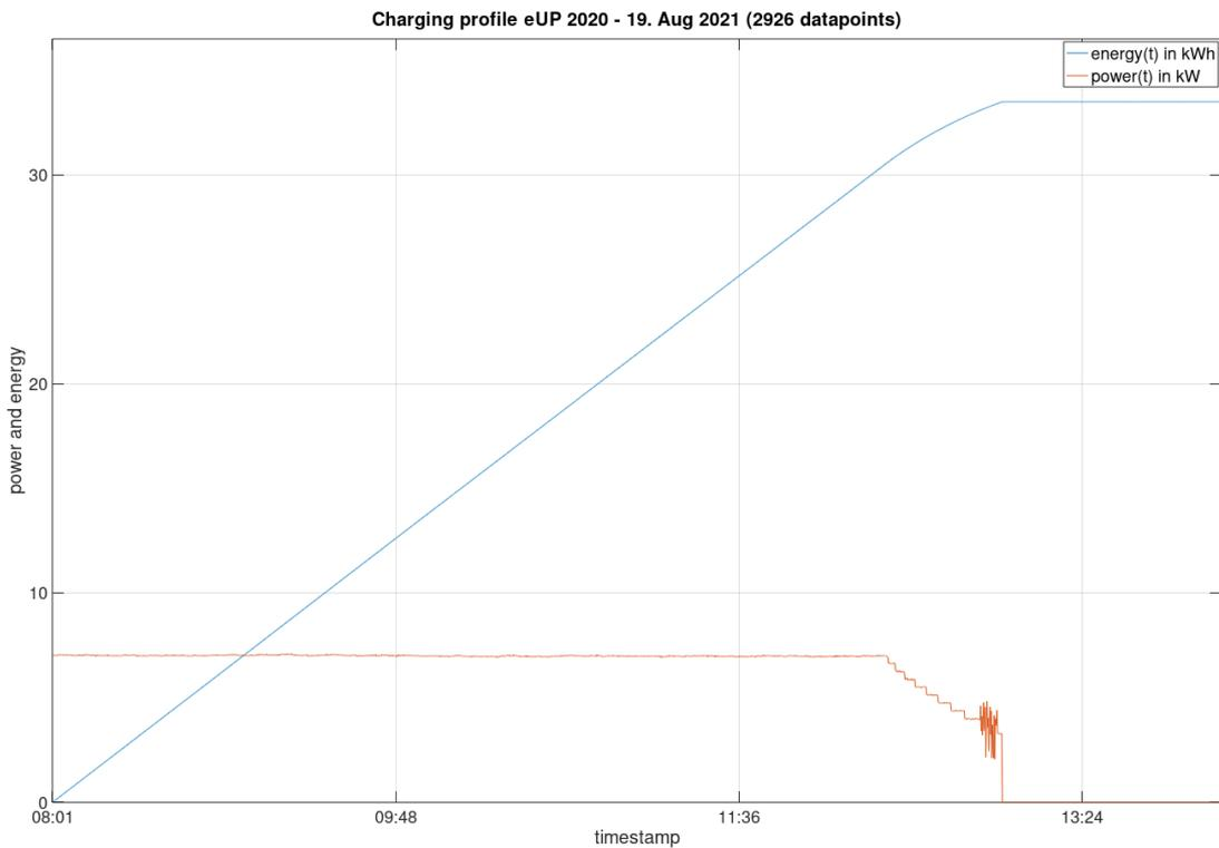
**Figure 7 – Charging profile of VW e-up!**
