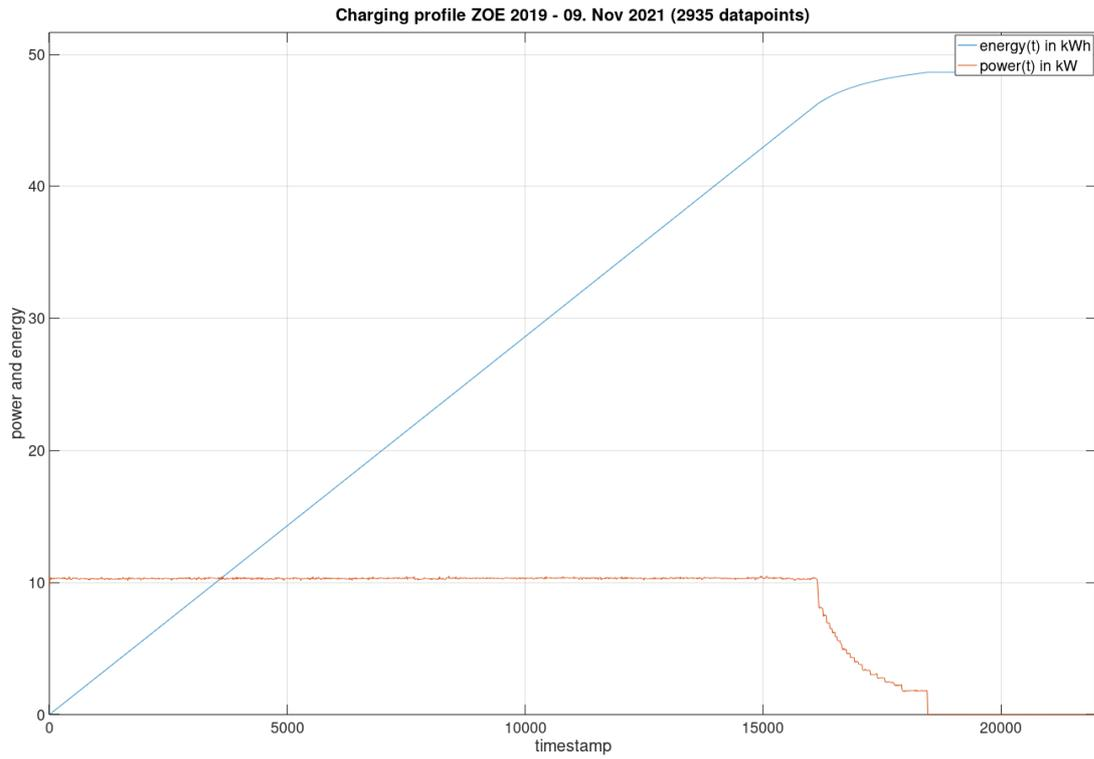
**Figure 6 - Charging profile of a Renault ZOE**
