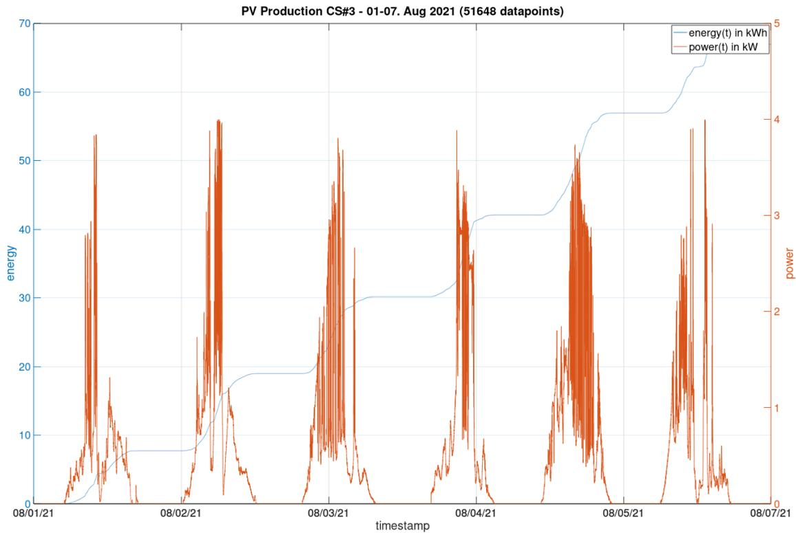
**Figure 12 – PV energy production chart from CS#3 (6 days)**
