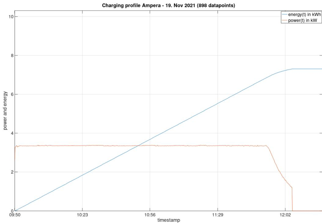
**Figure 9 - Charging profile of an Opel Ampera EV (built 2011)**
