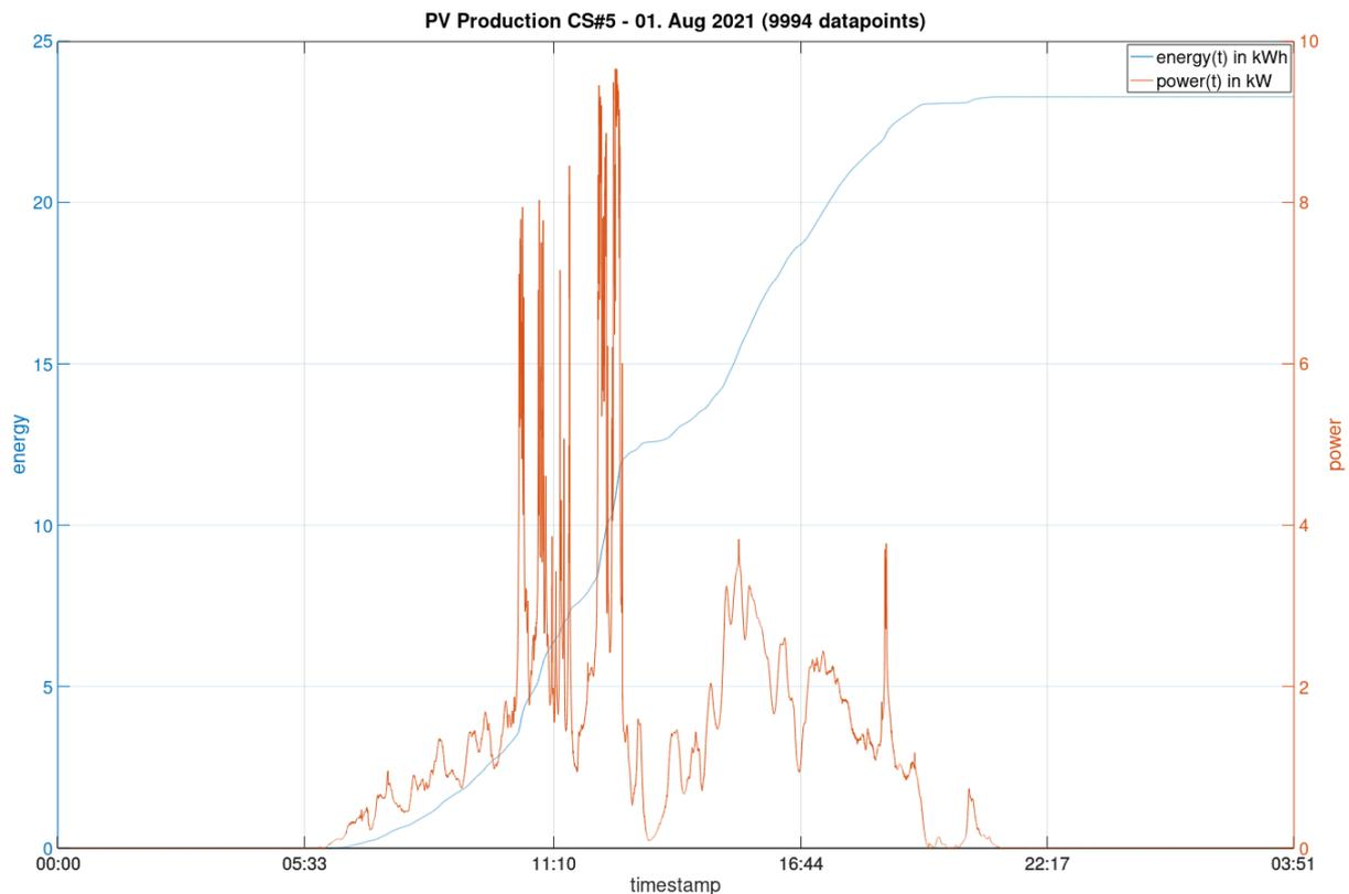
**Figure 11 - Typical day chart of PV energy production @CS#5 (01.08.2021)**
