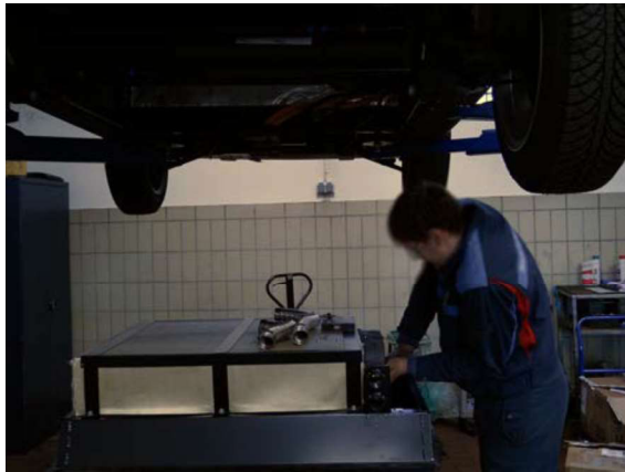
Figure 4: Extraction of the ZEBRA battery system
